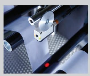
**FT 25-RA for dancer roll regulation** The precise control of the FT 25-RA ensures a constant tension of the paper roll during unwinding.
